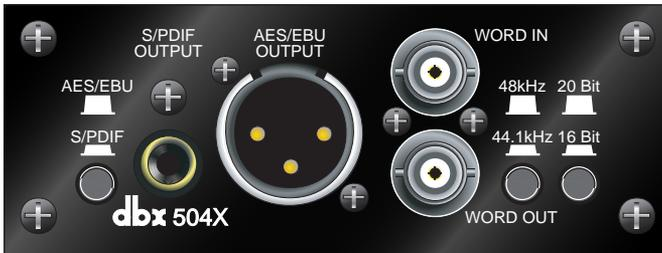
**AES/EBU / S/PDIF Switch:** Selects either AES/EBU format or S/PDIF digital output format.
