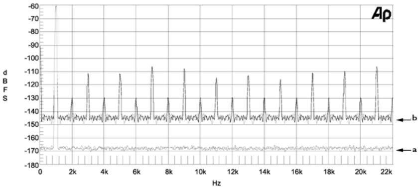
(a) 24-Bit word, (b) 16-Bit truncated output, no dither. Parameters: Input -60dBFS, 1 kHz; FFT Length= 2048, Sample Rate= 48 Khz, Averages= 32; Graph Steps= 1024.
