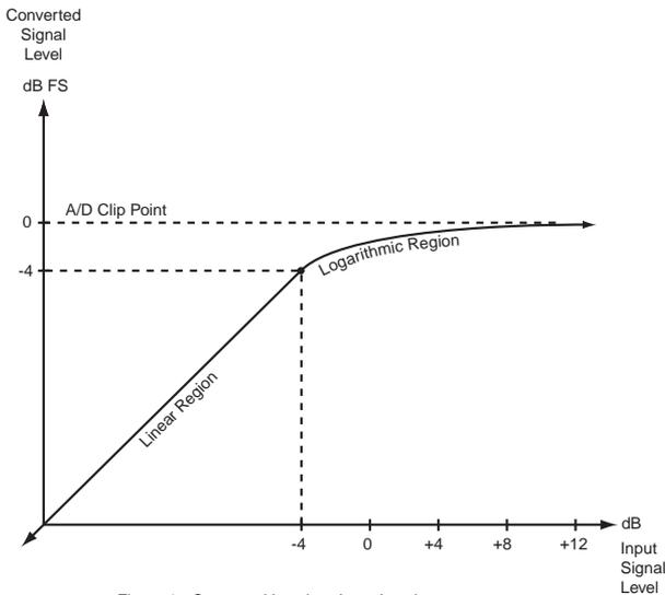
Figure 1 - Converted Level vs. Input Level
