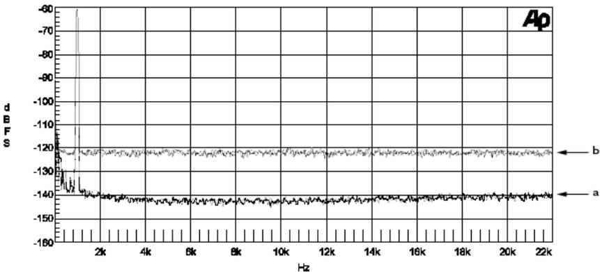
TPDF Dither. (a) 24-Bit word output, (b) 16-Bit word output. Parameters: Input - 60dBFS, 1 kHz; FFT Length= 2048, Sample Rate= 48 KHz, Averages= 32; Graph Steps= 1024.
