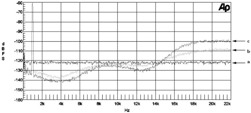
16-Bit TPDF dither. (a) Shape "off", (b) with shape set to "S1", (c) with shape set to "S2." Parameters: Input -60dBFS, 1 kHz; FFT Length= 2048, Sample Rate= 48 Khz, Averages= 32; Graph Steps= 1024.
