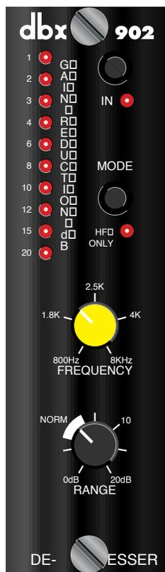
**GAIN REDUCTION LEDs:** Indicate the amount of de-essing in dB.
