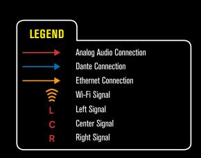
NOTE: For best performance, use CAT5e or higher straight-through Ethernet cables for Dante connections. See owner's manual for further information.
