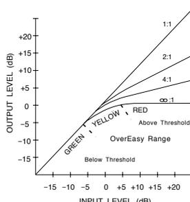
Figure 1: Hard Knee Compression Curve, and Threshold LEDs.
