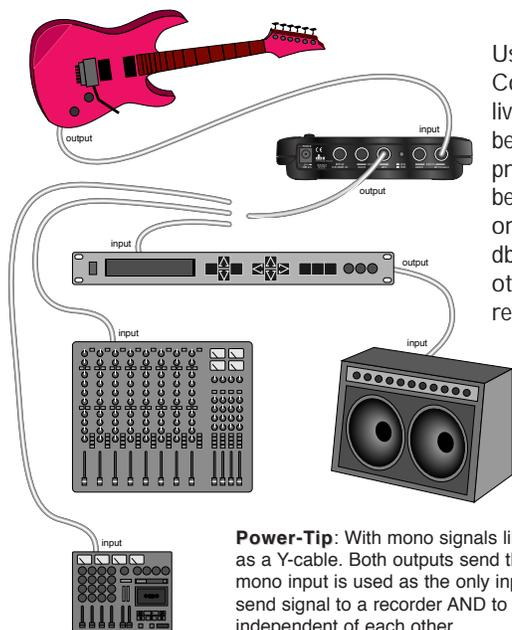
Use the dbx MC6 Mini-Comp™ Compressor in your live sound rig by putting it before your other signal processors. Or put it in line before you send to your mixer or recorder. Get that great dbx compression that no other guitar processor or recorder has!
