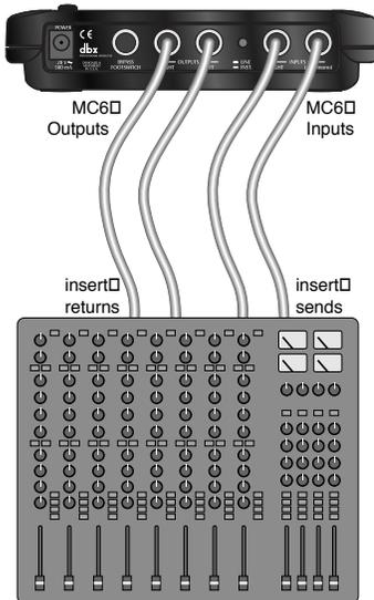
Use the MC6 to compress those pesky individual tracks by inserting it in the insert path of your mixer for a single channel or for a (stereo) linked pair of signals.
